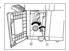
**5** Remove any paper misfed on the exit side of the saddle stitch unit.
